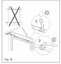
other directions. Lock the screws into place as shown in Fig. 12.
