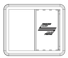
For better user experience, it is recommended to push Freezer Temperature Adjusting Slider to FRIDGE COLDER position, and turn the Refrigerator Temperature Controlling Knob to NORMAL position.
